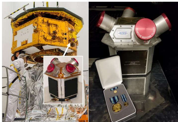
(L-R) Busek electro-spray thrusters aboard ESA LISA Pathfinder (credit: ESA); NASA Medal and four Busek ST-7 Electro-spray Thrusters (credit: Busek);
