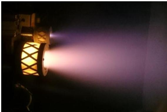
BIT-3 thruster and neutralizer firing on Xenon (top), Iodine (bottom)
