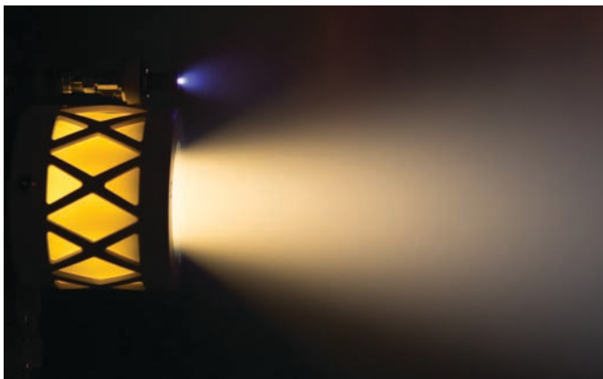
Busek has ground-tested an ion microthruster using iodine as a propellant, which has advantages for smallsats.
