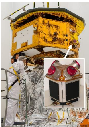
Busek electro spray thrusters aboard ESA LISA Pathfinder (credit: ESA)
