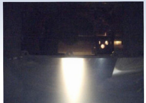
BIT-3 Flight Model Firing with Iodine Propellant
